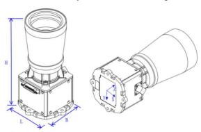
Note: The origin of the coordinates lies in the geometric center of the outer surface of the lower shell (see "Instrument diagram");
